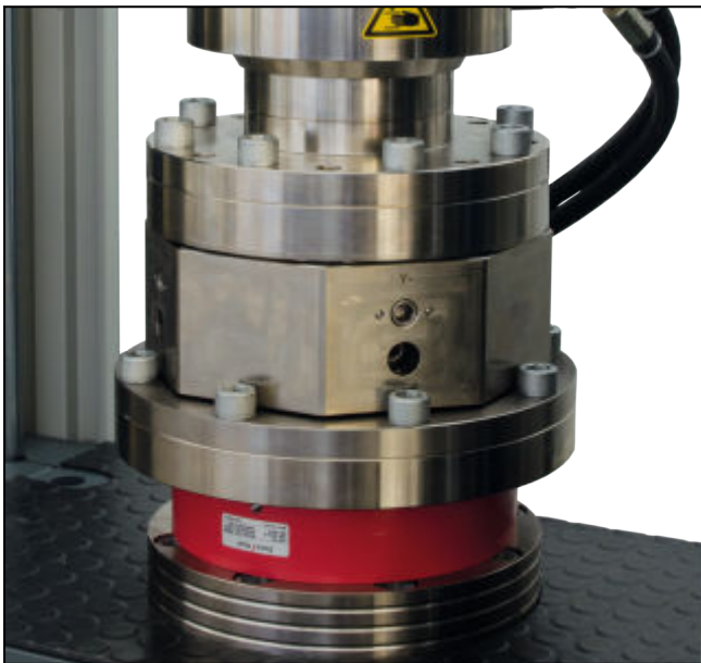
Alignment fixture Fmax 250 kN mounted between load cell and specimen grips via flange
